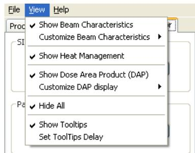
De-select 'Hide All', you can then choose 'Beam Characteristics', 'Heat Management' or 'Dose Area Product'. The screen can display all of these outputs at once if required; the 'Beam Characteristics' and 'Dose Area Product' outputs can be further customised.
