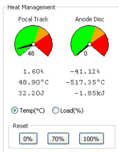
Once the exposure button is depressed (on the 'Exposure' tab) the heat is applied to the anode and dynamic cooling occurs, in real time, showing the effect of repeat exposures.
